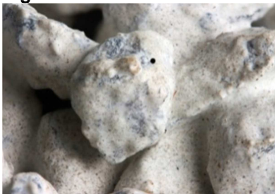
Figure 5 - A composite Close Up of a Permeaccrete Showing Carbonate Bridging
