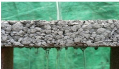
Figure 6 - A Permeaccrete Showing Water Passing Through
